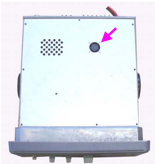
Fig.3 PA Cooling Fan in the upper shield plate
