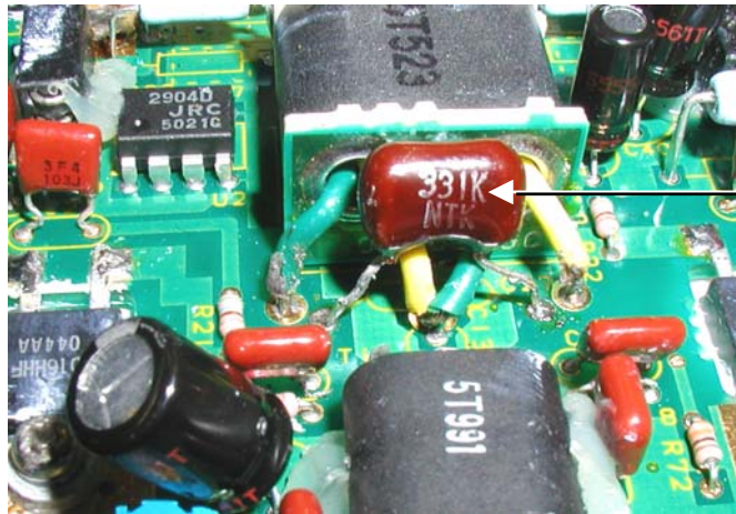
Fig.1 C27, 330 pF on 05P0667 with 2SC2879A
